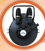
Single Phase 2 Motor Australian certified H-Class Dust Extractor. It is equipped with a washable M Class Primary filter and two H Class certified H13 filter. Each H13 HEPA filter is individually tested and certified to have a minimum efficiency of 99.99% at 0.3 microns, which meets the Australian silica dust control requirements. This professional dust extractor is designed for control of all types of dust from building, grinding, cutting and drilling concrete substrates.
